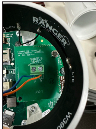
Figure 14: Blue (B-) Wire into B slot, Orange (A+) Wire into A Slot
