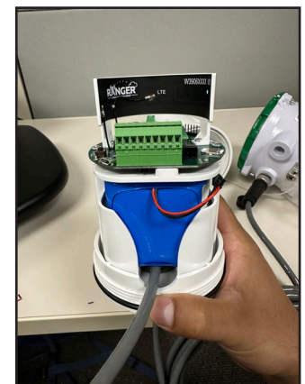
Figure 11: Circuit Board Module Installed without Power and with Cable Underneath
