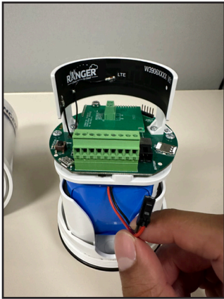
Figure 5: Ranger with Battery Power Cable Removed
