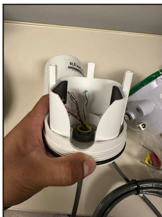
Figure 9: Cable Fed Through Central Hole in Ranger
