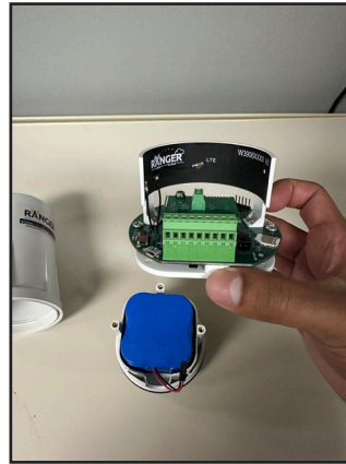
Figure 7: Ranger with Battery Power Cable Removed
