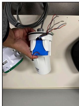
Figure 10: Battery Installed with Cable Underneath
