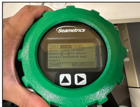
Figure 17: COMM Menu on Seametrics AG90, with Baud Rate Set to 19200 and No Parity Bit
