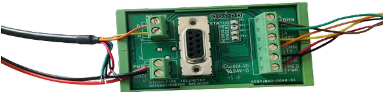
Figure 6: SignalFire Breakout Dongle interface
