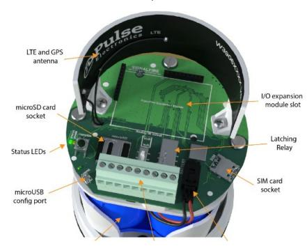
The Ranger cellular transmitter comes complete with a web- and mobile-friendly SignalFire Cloud interface, which allows users to remotely monitor assets, view trends, and receive alarms either by text or email. It also provides for remote configuration and troubleshooting of the Ranger node and the sensor to which it is attached.
