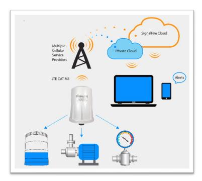
The Ranger powers the sensor and publishes data to the SignalFire Cloud so users can monitor and trend tank levels and receive email/text alarms.
