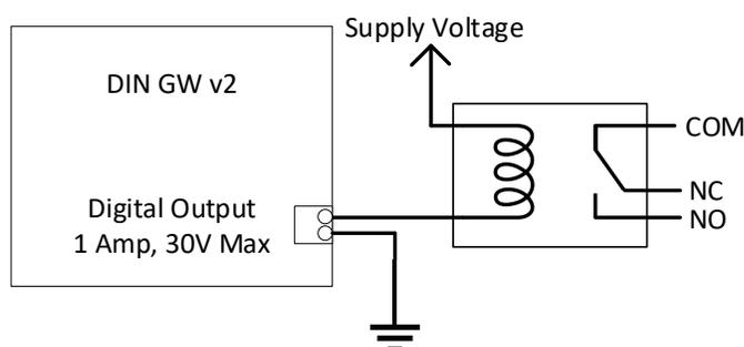
Note: The digital outputs on the gateway have built in protection and can drive relays and inductive loads directly.
