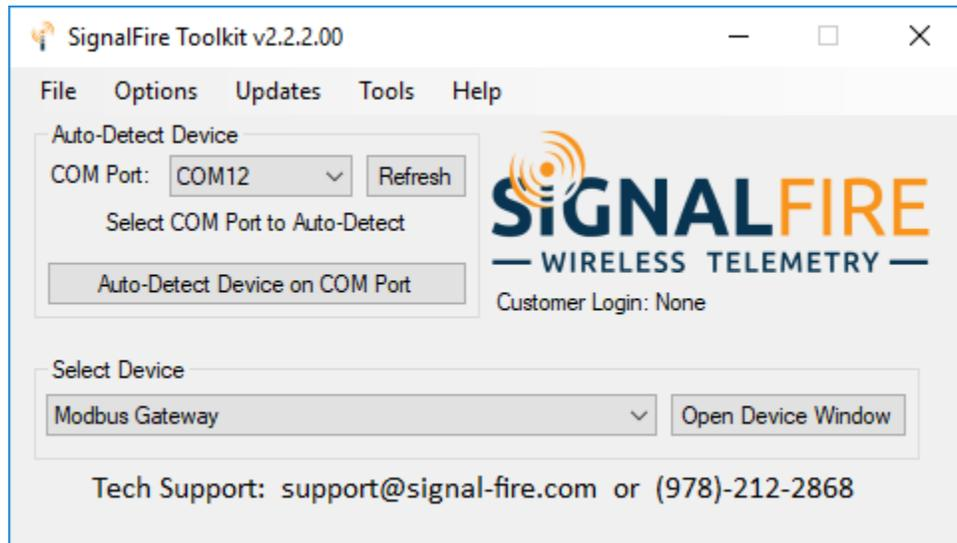
Select the COM port associated with the DIN Gateway and click “Auto-Detect Device on COM Port.” This will open the device configuration window, where all device settings can be configured.
