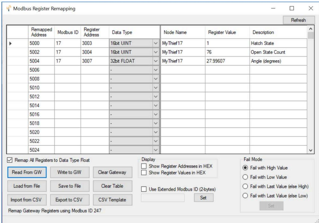
For each even numbered register address in the remap table, enter the Modbus ID, Register Address, and select the data type. The data types are provided in a pull-down list. Click **Write to GW** to remap the register(s).
