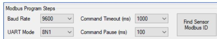
Control the sensor power as described in section [SENSOR POWER CONTROL](#), select a limited search range or search the entire Modbus ID range (1 to 31), then click **Find**.
