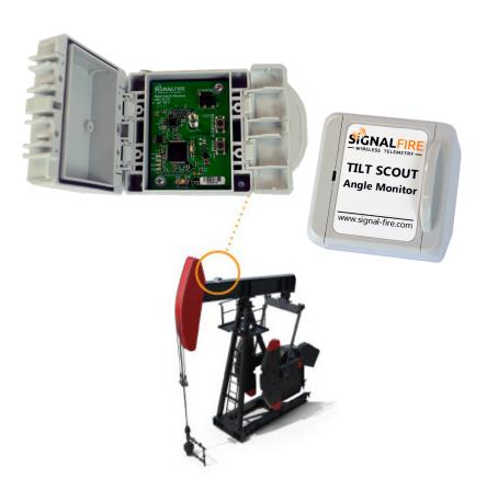
Instead of wiring sensors to the pump jack as part of a remote monitoring and control system, the TiltSCOUT magnetically attaches to the pump jack without any tools. Operators simply hand-mount the unit in any orientation, calibrate the zero position with a local push-button, and the unit checks in with the Gateway automatically.
