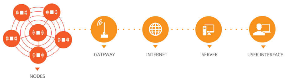
Graph 1: SignalFire's remote sensing system consists of remote nodes that wirelessly power and extract data from sensors for transmission to a gateway that links to the internet and back-end servers in bringing tank level data to a control center or PC
