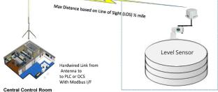
Shown is a single tank configuration outlining how the Sentinel node interfaces with the level sensor in transmitting data to a Gateway that ties into a PLC within a central control room. All transmission distances are based on good line of sight.
