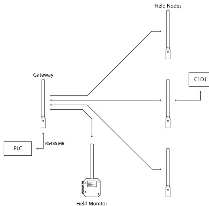
The field Nodes are sending their data to the Gateway where it is being read by a local PLC. The Field Monitor is positioned so that it can communicate with the Gateway, and when the button is pressed, it contacts the gateway and downloads the relevant data that it needs to display the configured register data.
