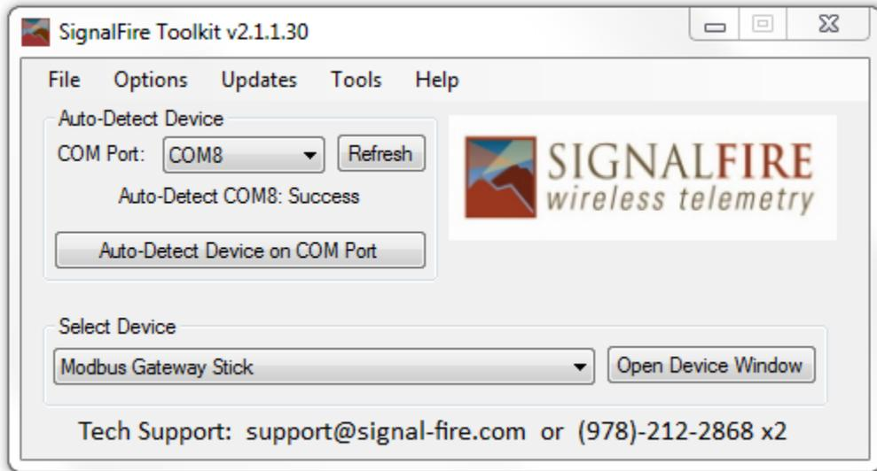
Select the COM port associated with the Field Monitor and click "Auto-Detect Device on COM Port." This will open the device configuration window, where all device settings can be configured.
