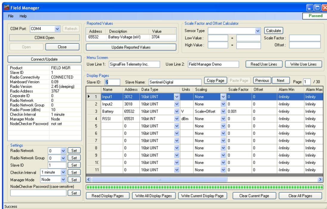
In the example above, the Field Monitor is configured to show the digital input state for both channels of the Sentinel Node along with the battery voltage and RSSI of that node. Each line of the display must be given a name of up to 8 characters. Each line may also optionally be given a tag of up to 4 characters.
