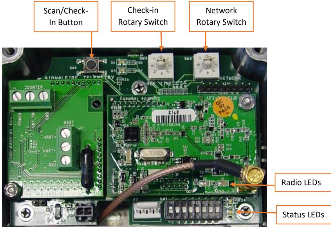
**Note: the rotary switches and DIP switch are only installed on legacy devices. All new devices are shipped without the rotary and DIP switch and all configuration is done with the ToolKit.**
