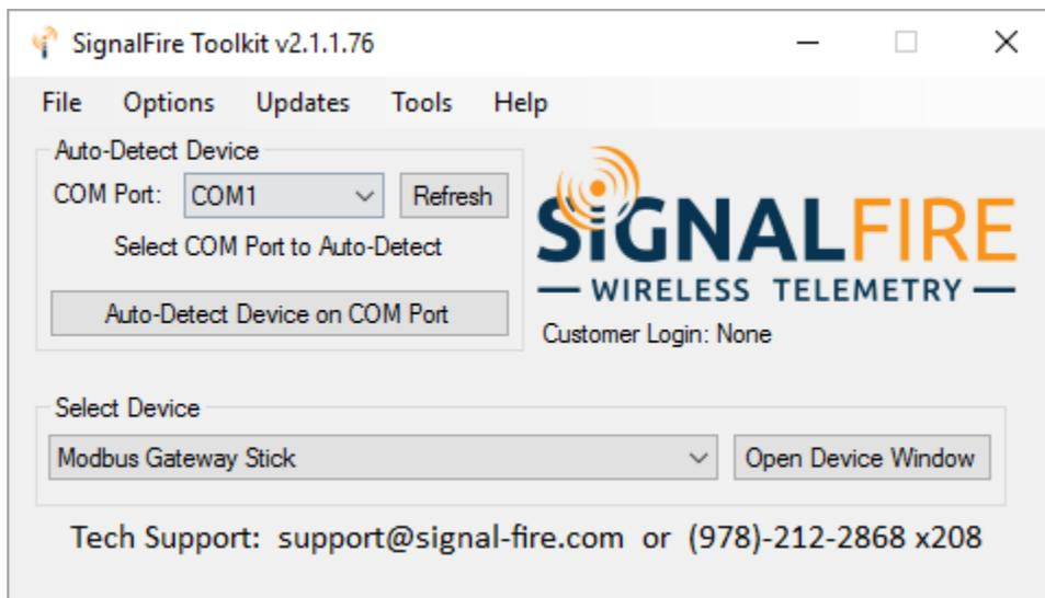
Select the COM port associated with the A2 Node and click "Auto-Detect Device on COM Port." This will open the device configuration window, where all device settings can be configured.
