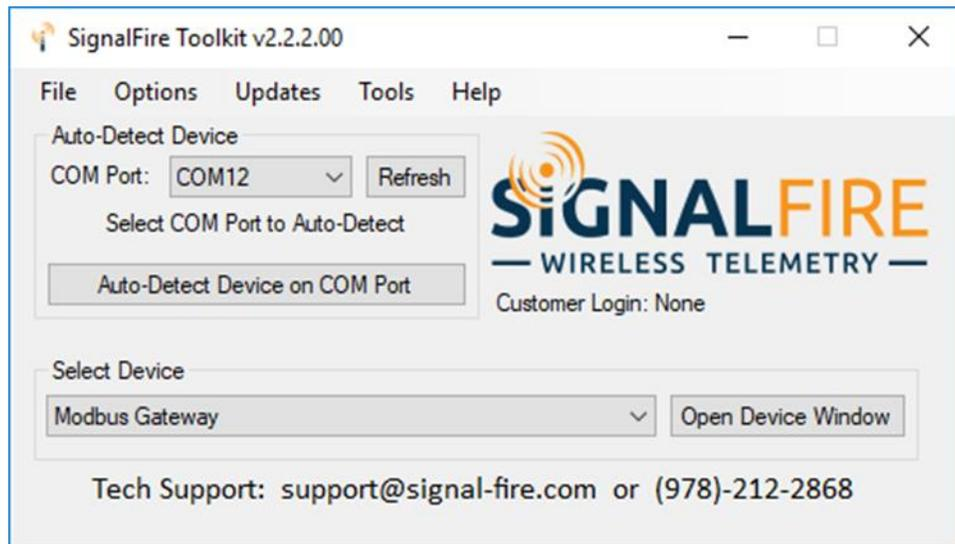
Select the COM port associated with the Sentinel Node and click “Auto-Detect Device on COM Port.” This will open the device configuration window, where all device settings can be configured.
