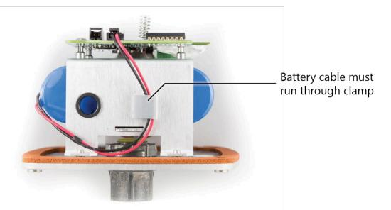
Plug the internal lithium battery pack into the connector labeled LITHIUM BATTERY as show below. Be careful to insert the battery connector as pictured with the locking tab facing up.
