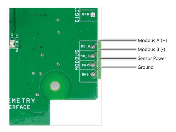
The Sentinel Modbus node has a single terminal block for connection to a Modbus sensor.
